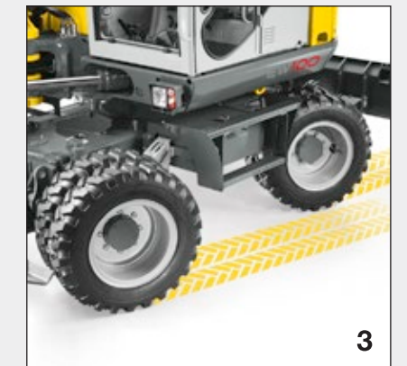
Crab steering for parallel travel, e.g. along buildings.
