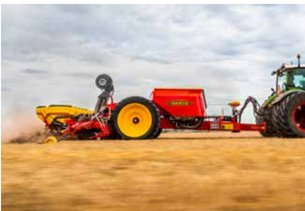
A 3000 litre fertiliser hopper is available as a compliment to the 5000 litre hopper on the top-capacity models.
