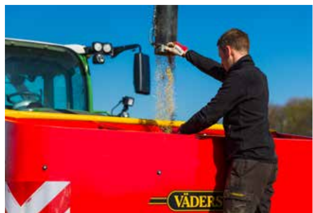
The sloping front design gives the driver good visibility. The wide opening and built in step makes it easy to fill.
