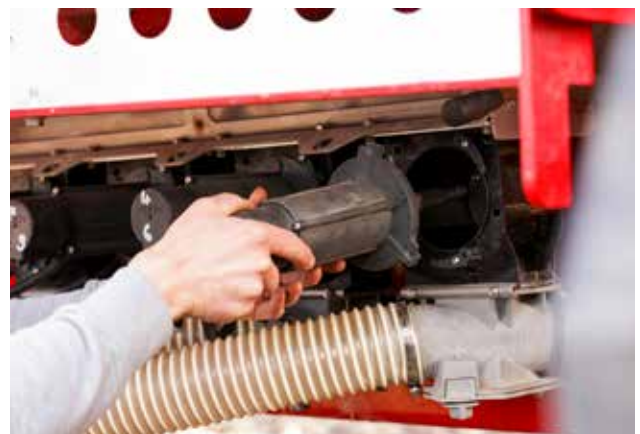
The fertiliser is metered via the high-capacity metering system, Fenix III, with a capacity up to 350kg/ha at 15km/h.
