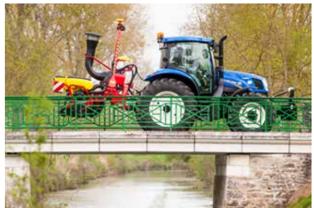
The 3 metre wide Tempo R is mounted on the tractor's three-point linkage, making it easy to manoeuvre in the field.
