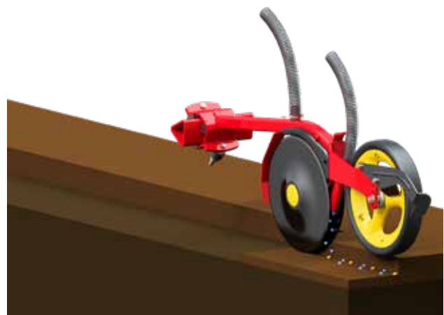
The InLine version places the fertiliser in a separate outlet together with seeds in the seed coulters.
