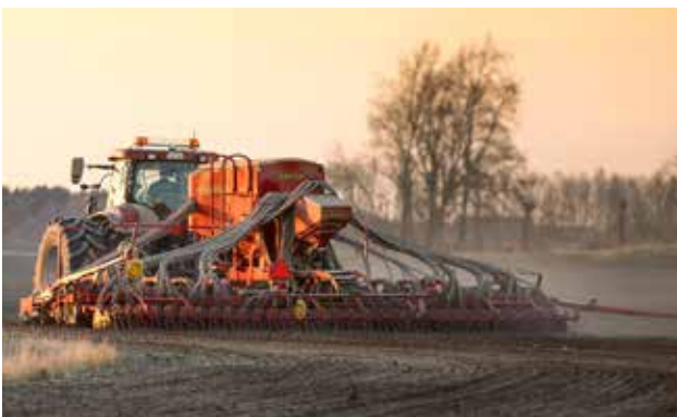
To optimise the output on the field, Spirit 600-900C is equipped with half machine shut-off for both the seed and fertiliser.
