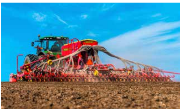
Spirit 600-900S enables the driver to conduct half machine shut-off directly from the driver seat.
