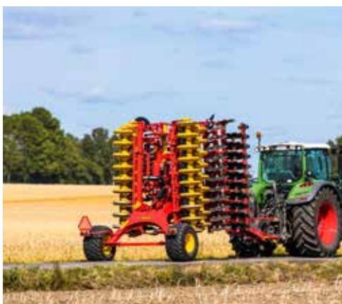
When transporting Carrier XL 425-725 between fields, the machine is wing-folded to fit within 3m transport width.
