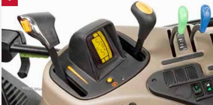
**2** cotiera de control avansat la tractoarele Maxxum Multicontroller™ echipate cu transmisie ActiveDrive 8.
